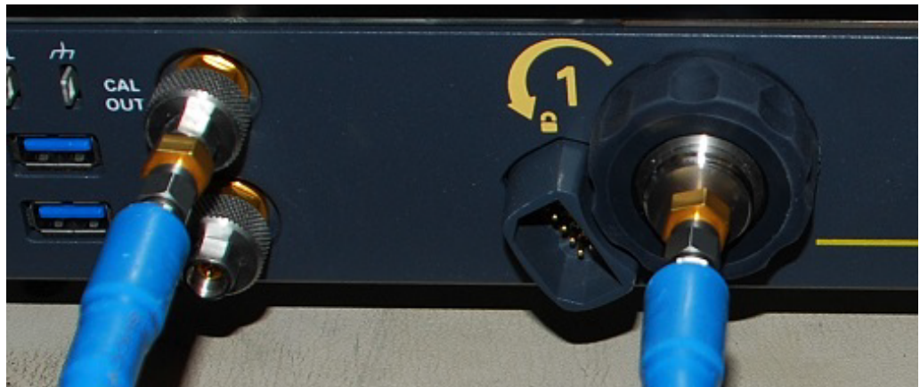
Figure 13 Verifying basic oscilloscope operation -- models with 3.5 mm input connectors
